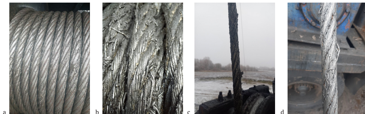
Figure 2. Appearance of the drilling line with signs of fretting damage and destruction of the wires of the drilling line of the UPA-60X unit
