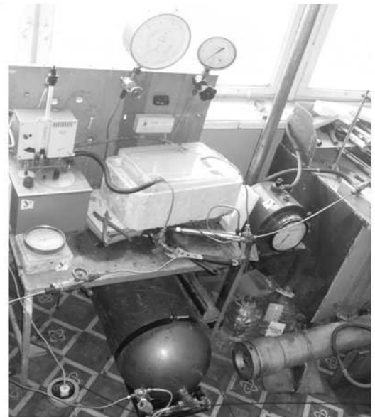
1 – model; 2 – source of gas; 3 – reference cell; 4 – pressure gauges; 5 – manifolds; 6 – input valve; 7 – output valve; 8 – вакуумний насос; 9 – gas meter; 10 – thermo bath; 11 – temperature sensor
