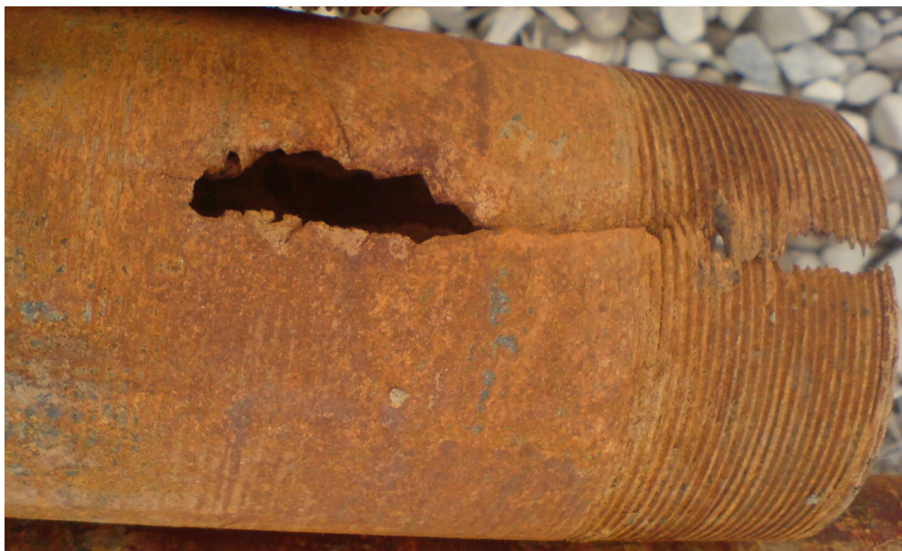
Figure 2 – State of the 139,7 mm flow tubing borehole № 59 Pivnichna Dolyna
